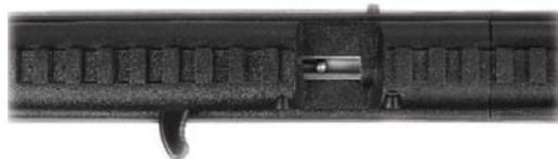
A magnet holds each BB in place.
